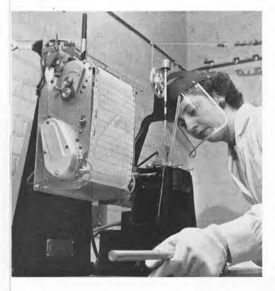
Operating a gadget which determines the viscosity of molten plastics at the temperatures they will be molded into pen parts is a tricky assignment. Eileen V ander bloemen handles it well.
